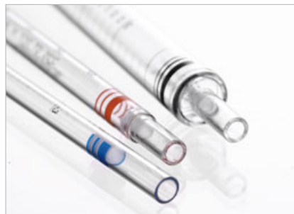
With filters, different colors correspond to different volumes
