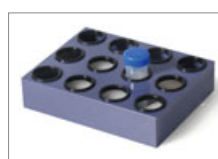
Standard plate: Height 45mm. O-ring well included: Ø33×12
