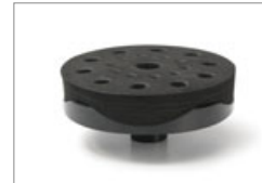
Multi-well plates, for 1.5mL and 2mL Micro centrifuge tubes.
